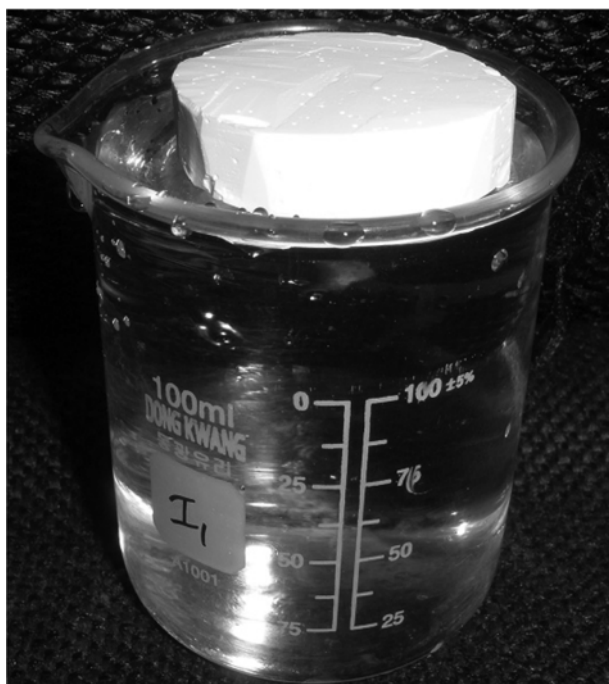
Fig. 6. The monolithic hydrophobic silica aerogel floating on the surface of water.
